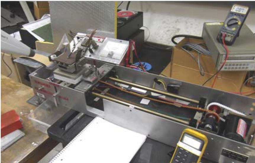
**Overview of the HCOF set-up showing the sled chain drive, sled and base, heater and load controls electronics.**
