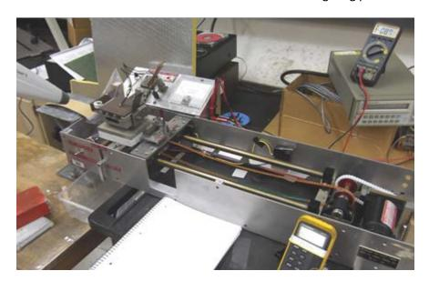
Overview of the HCOF set-up showing the sled chain drive, sled and base, heater and load controls electronics.
