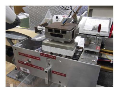
Close-up of the HCOF sled and base, a test strip is adhered to a clamped Mylar strip and pulled to the right through the heated sled/base assembly. Steam from a portable steam cleaner is applied to the paper test strip at the point prior to entering the sled/base area.
