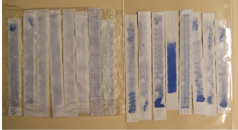
Figure 4. Underside of the inked strips shown in Figure 3 displaying varying degrees of show-through.
